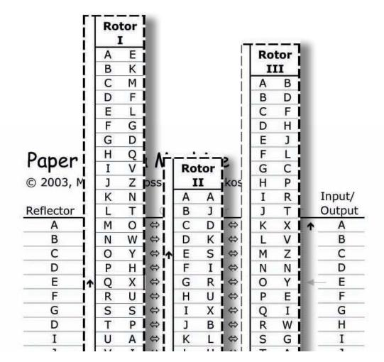
2. The first step of encoding any letter is to *Advance the Rotors*. This is done before encoding each letter – even the first one. The right-most rotor is always shifted up one letter. So, in our example, rotor III is shifted up to the "L" position.
